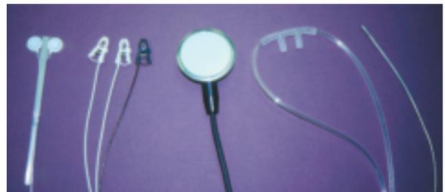
*System transducers include (from left) tongue array, EMG electrodes, stethoscopic microphone, nasal cannula, and solid state manometer. Two auxiliary channels are provided for other signals of interest.*
